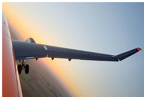
Figure 17. Small-scale demonstrator in flight with flapping wing tips (AlbatrossONE).
