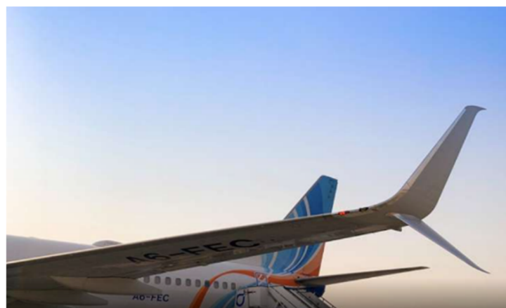
Figure 13. Split scimitar fitted on Boeing 737-800 [82].
