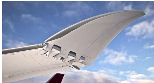
Figure 16. Folding wingtip device (Boeing 777X).
