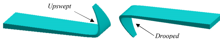
Figure 15. Upswept and drooped wingtips (reproduced from [84]).
