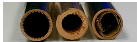
Figure 15. Axial groove, mesh, and sintered cross-section [56].
