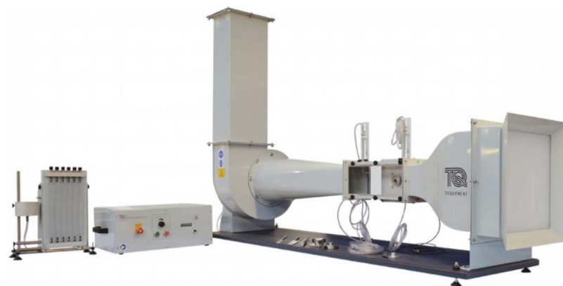
Figure 3. The AF-1125 low-speed wind tunnel of NUAA's AEEA group.
