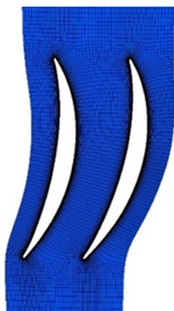
Figure 3. Fluid domain mesh for Rotor 67 blade at near hub location.
