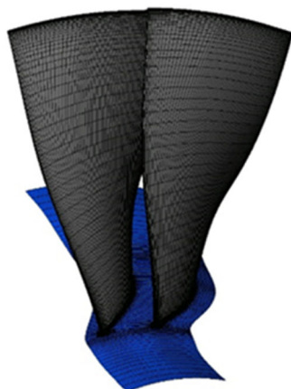
Figure 4. Fluid domain mesh for Rotor 67 for blade.
