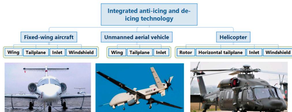
Figure 2. Analysis of application scenarios for integrated electrothermal anti-deicing function structures in aircraft.
