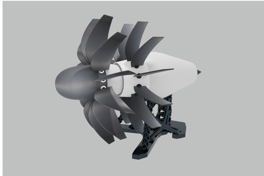
Figure 1. The new-generation open-rotor engine configuration.
