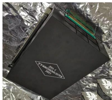
Figure 2. A photo of the space environment monitoring unit.
