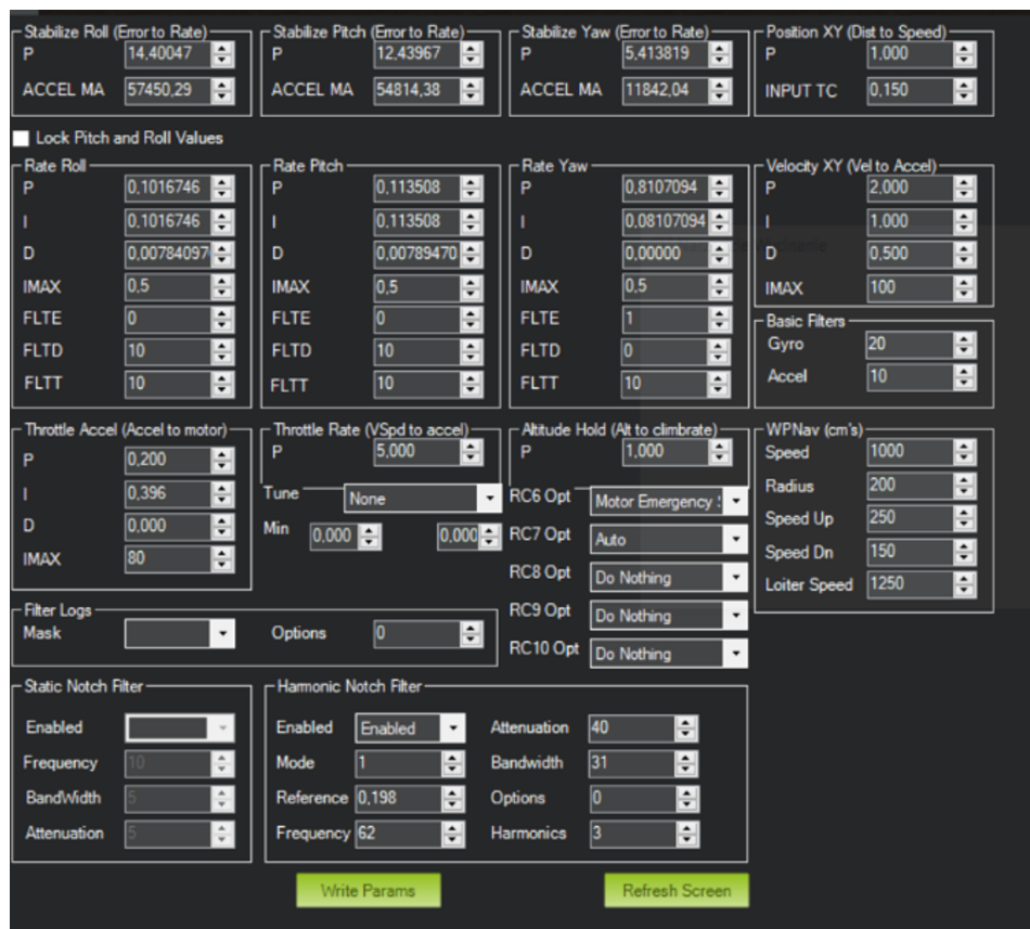
Figure 10. Tuning of PID and autopilot parameters in MissionPlanner.
