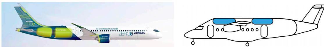
**Figure 3.** Examples of hydrogen tank integration in fuselages: without airframe modifications ((left), image adapted from [56]), and with fuselage modification ((right), image adapted from [57]).
