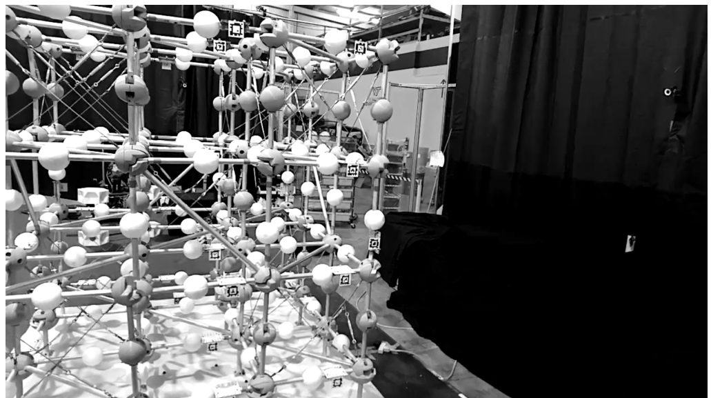
Figure 25. Camera view of the inspection test after the completion of the BORG truss assembly.
