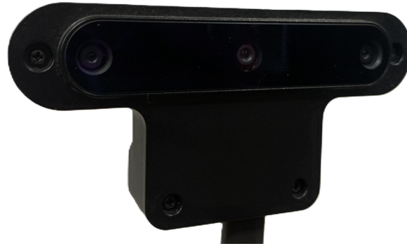
Figure 8. Oak-D stereo camera used for hardware testing to collect video for AprilTag detection.
