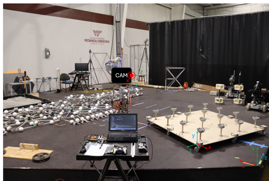
Figure 14. Lab space with coordinate frames for the camera, AprilTags, and OptiTrack origin.
