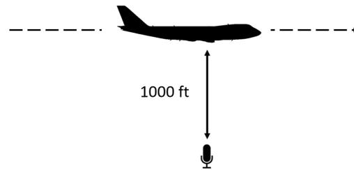
**Figure 2.** Schematic representation of the moved-along receiver located 1000 ft vertically below the aircraft.
