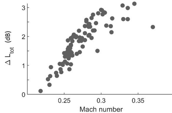
**Figure 7.** Difference of sound pressure level ( $\Delta L_{\text{tot}}$ ) for a moved-along receiver (1000 ft underneath the aircraft) caused by landing gear extension for an Airbus A321.
