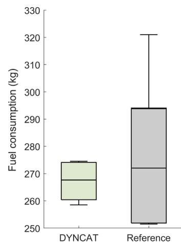
**Figure 4.** Boxplots of fuel consumption of flights with (green) and without (grey) using DYN-CAT.
