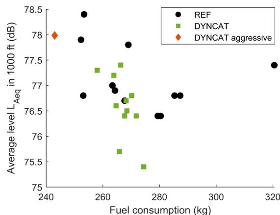
**Figure 8.** Fuel consumption vs. energetically averaged sound pressure level (at 1000 ft distance over 10–3 NM to runway threshold), compared for reference (REF) and DYN-CAT flights.
