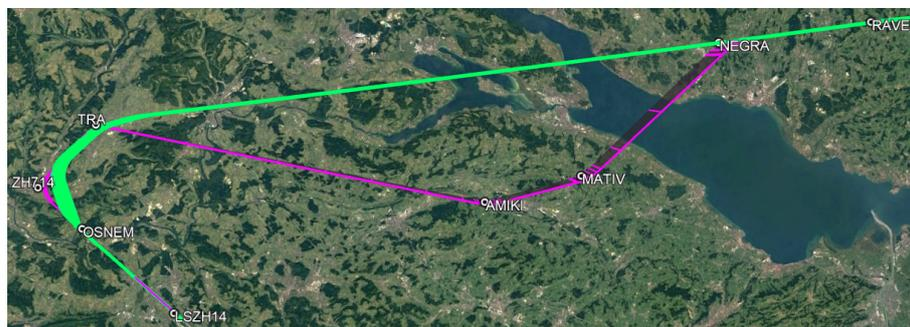
**Figure 1.** Planned flight track according to the flight plan (magenta) and actual flight track (green) after ATC instruction (short-cut to waypoint TRA). Credit: Google Earth.
