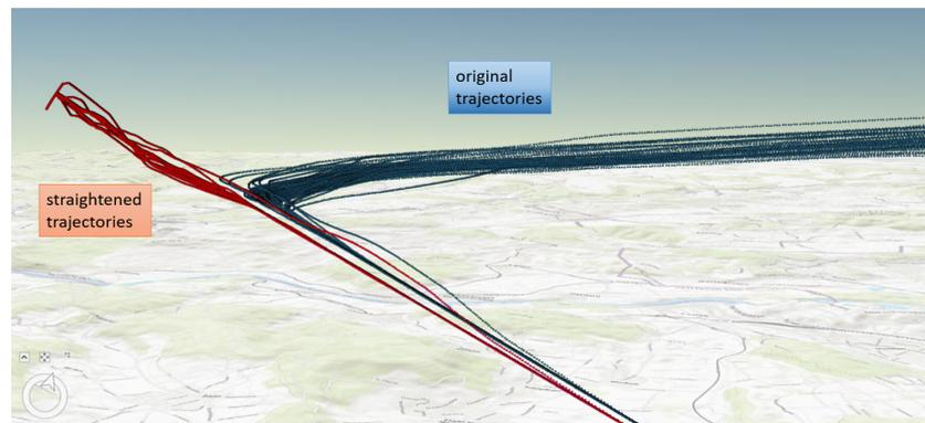
**Figure 3.** Original and straightened trajectories of all trial flights in blue and red, respectively. Credit: ArcGIS Pro.
