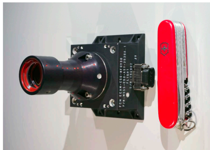
Figure 10. Image of a previously constructed Malin Space Science Systems (MSSS) ECAM camera that is identical to the CCRS vision system camera design.
