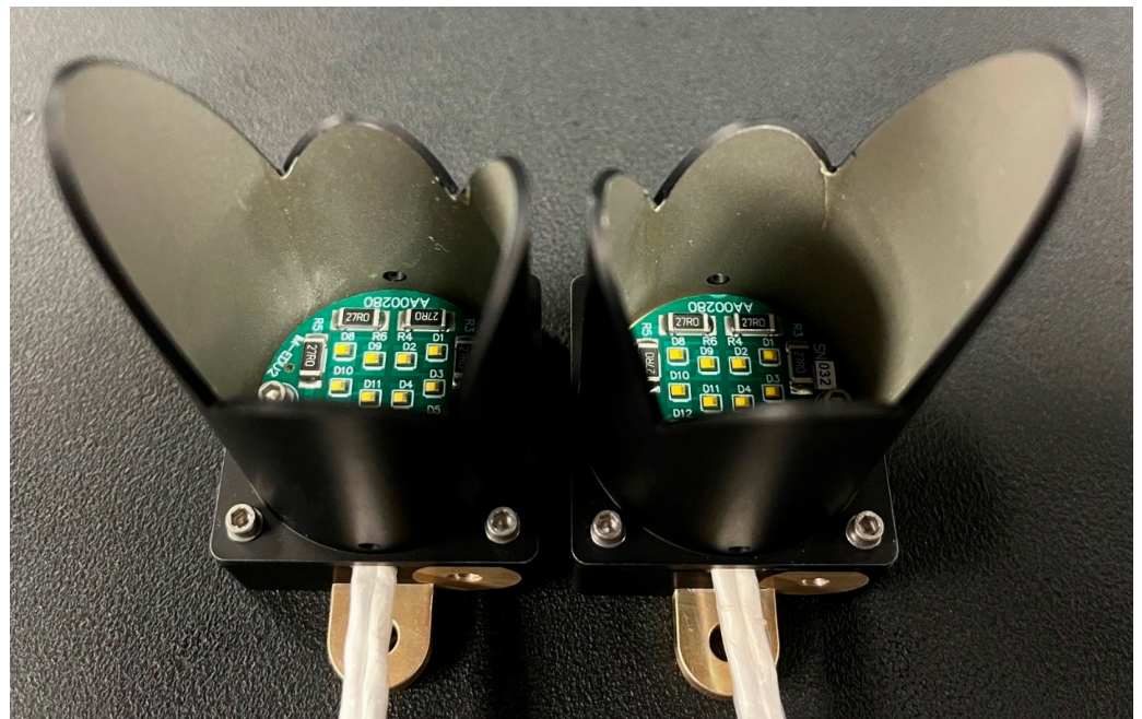
Figure 29. Image of two of the EDU illumination modules constructed from the flight model design. Although the -Z module (left) and the +Z module (right) baffles appear to be mirror copies, they are not exact mirror matches due to the use of a common module base. The small hole visible near the PCB in each module is for EDU test instrumentation and will not be present in the flight models (Photo Credit: Katherine M. Mellos).
