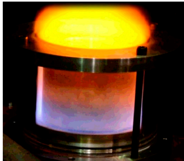
Figure 6. Optically accessible RDE model [29,30].
