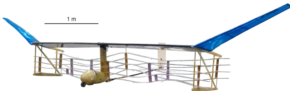
Figure 2. Photograph of the actual EAD aircraft tested by MIT, including its high-voltage power converter and EAD thruster.
