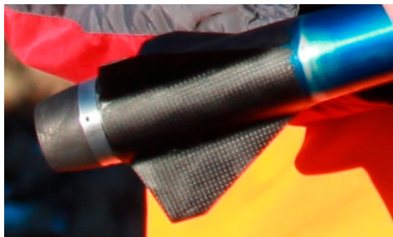
Figure 1. Milly—Tail fins and tapered tail cone containing graphite expander.
