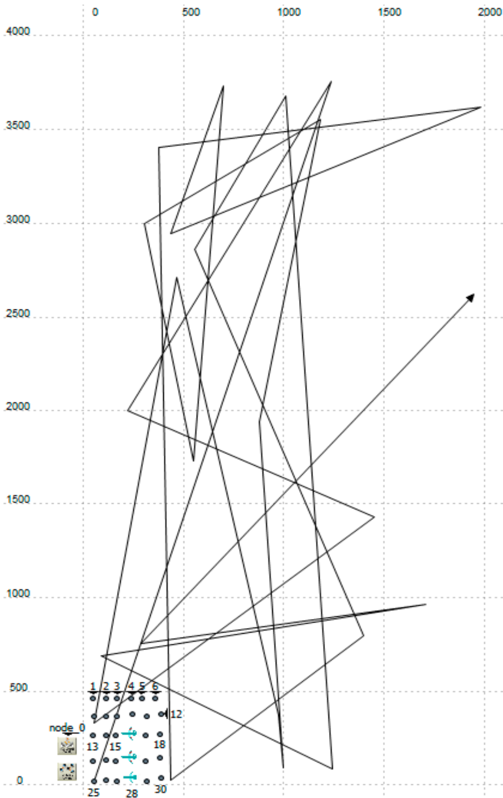
Figure 1. Trajectory of a UAV under the random waypoint (RWP) model.
