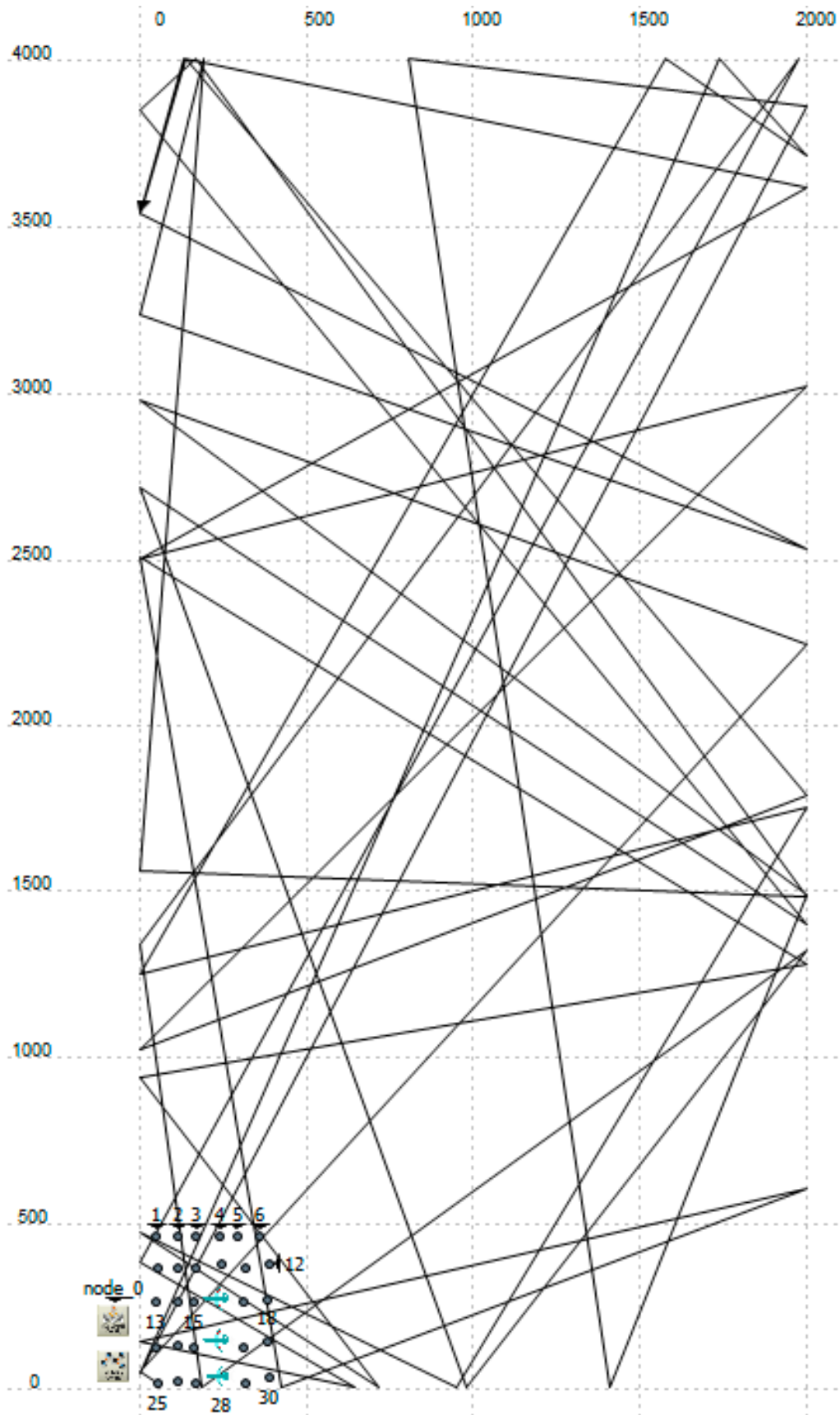
Figure 2. Trajectory of a UAV under the random direction (RD) model.
