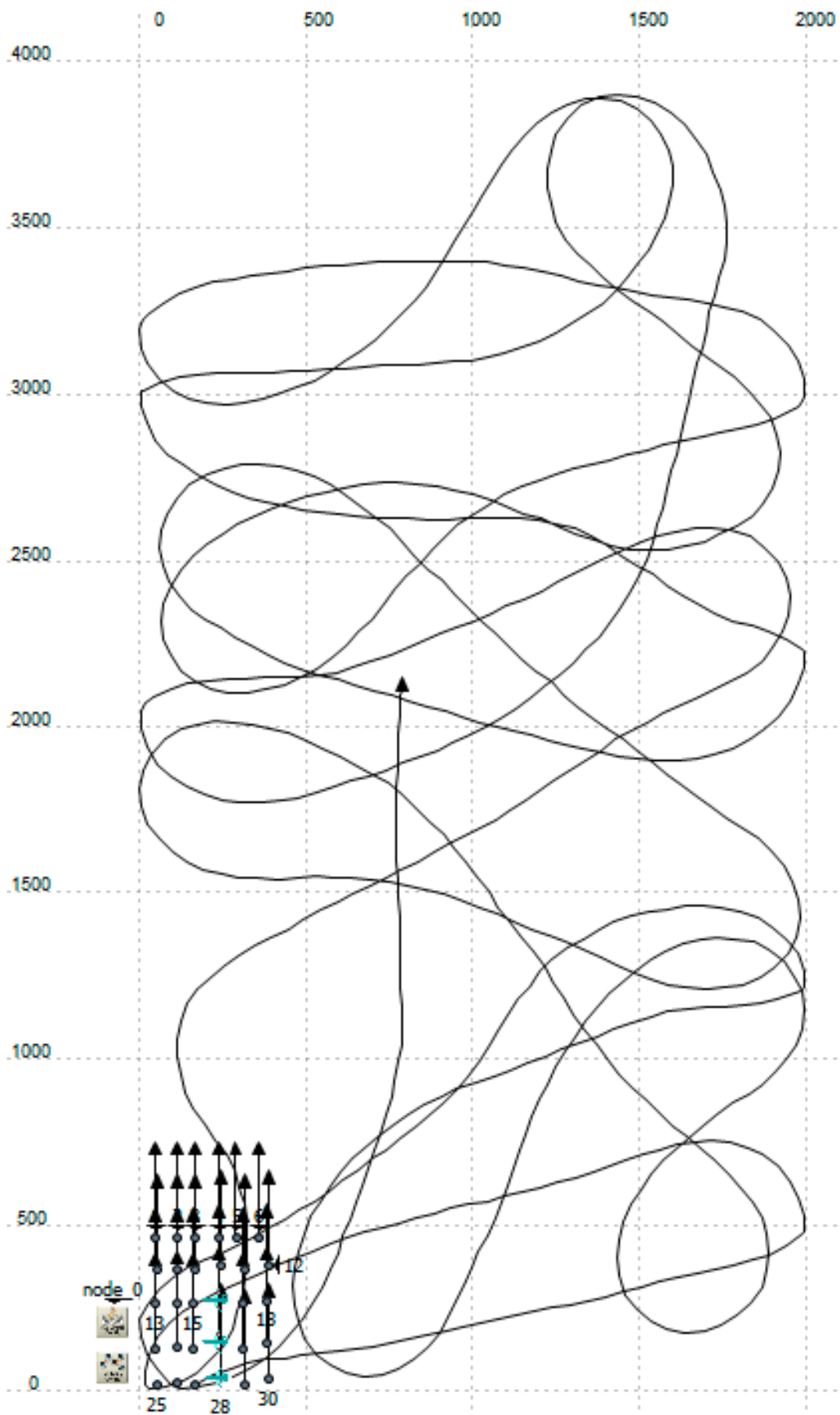
Figure 5. Trajectory of a UAV under the enhanced GM (EGM) model.
