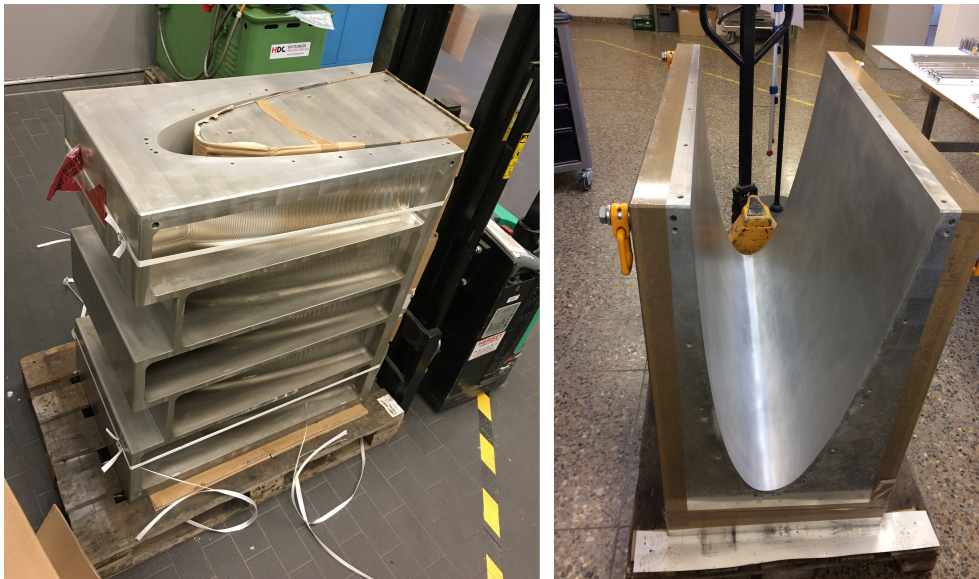
Figure 6. Photographs of the main aluminium negative mold after the wire electrical discharge machining (EDM) process and removal of the inner positive mold.
