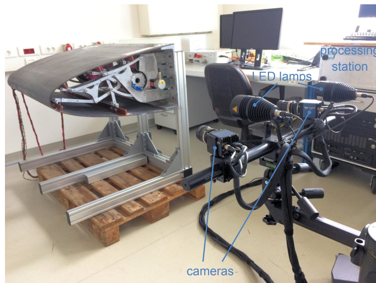
Figure 10. Photograph of the ARAMIS digital image correlation measurement setup for tracking kinematic and stringer trajectories.
