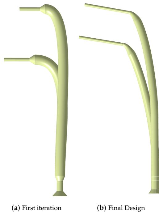
**Figure 7.** Evolution of the tube wall geometry during leakage optimization.
