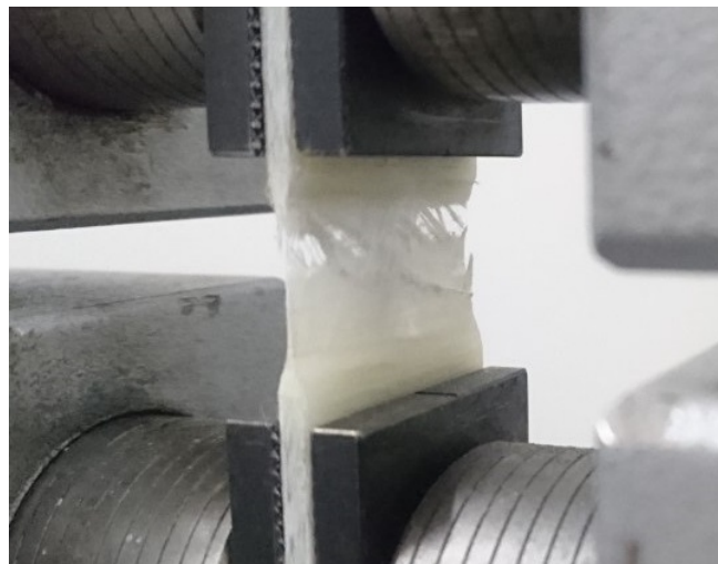
Figure 18. Failure of flexure hinge specimen at tensile test.
