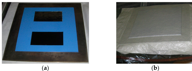
Figure 6. Bistable laminates manufacturing: (a) Hexply 8552 prepregs on the mold and (b) vacuum bag.
