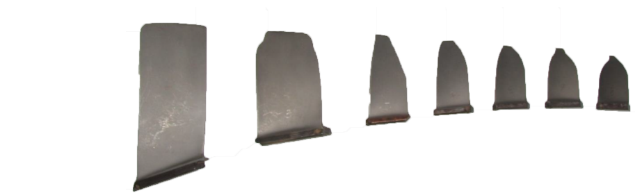
Figure 2. Erosive wear of compressor blades.
