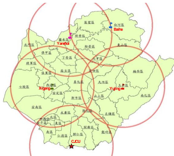
Figure 3. Long range wide area network (LoRa) ground transceiver station (GTS) deployment in Tainan for the first proof of concept (POC).
