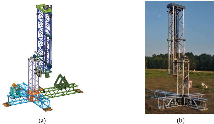
Figure 20. (a) The 3D CAD model of the launcher; (b) the launcher fully deployed before flight tests.
