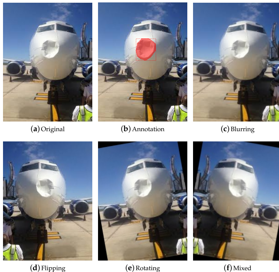
Figure 3. Example illustrating how the selected augmentation techniques preserve the dents in the image.
