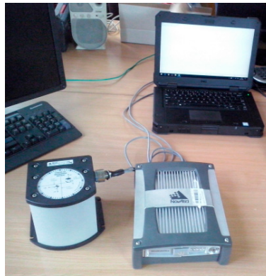
Figure 6. LN200 inertial measurement unit during static testing.
