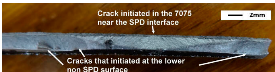
Figure 20. Multiple initiation sites both on the repaired (coated) side, in the 7075-T6 near the interface with the coating, and on the opposing face that did not have a coating.
