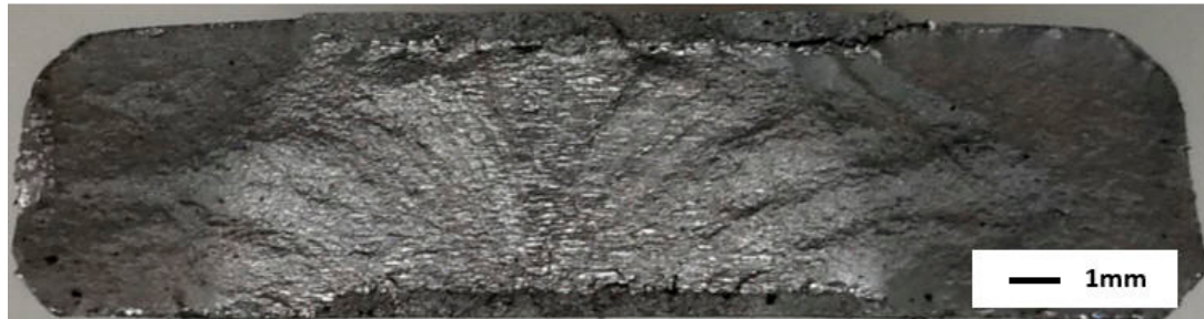
Figure 14. Failure surface associated with specimen 6061_F_2, failed at 87,958 cycles.
