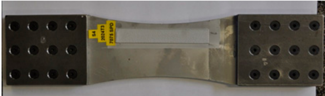
Figure 22. Location of the 7075 SPD strip on the 2024-T3 specimen.
