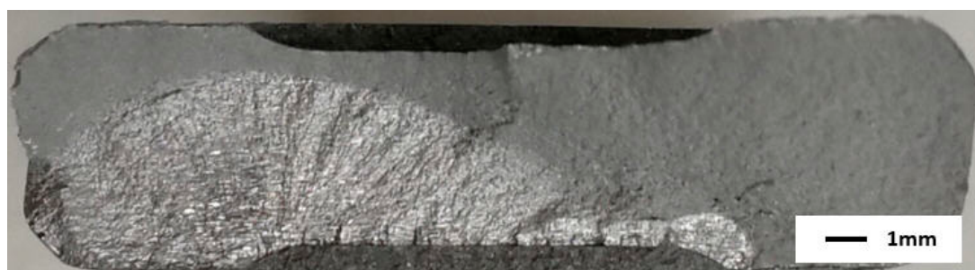
Figure 17. Failure surface associated with AMC LT-NGB 1, failed at 54,801 cycles.
