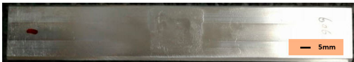
Figure 12. A specimen repaired with a 6061 powder coating.
