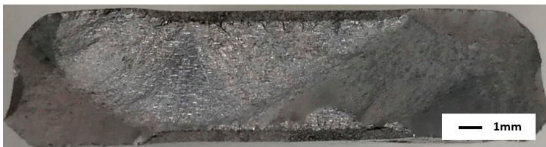
Figure 15. Failure surface associated with specimen 7075_F_3, failed at 83,590 cycles.
