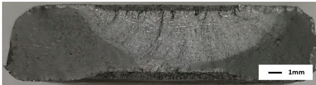
Figure 18. Failure surface associated with specimen 7075HT_F_1, failed at 36,284 cycles.
