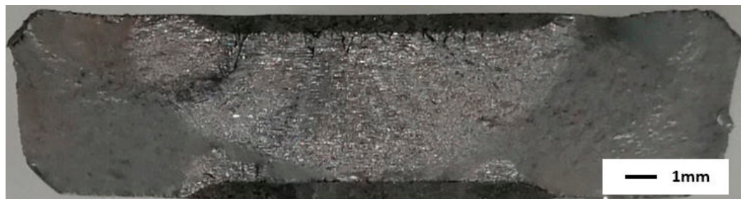
Figure 16. Failure surface associated with specimen AMC_F_1, failed at 38,677 cycles.
