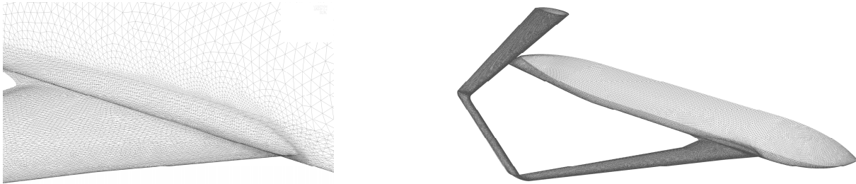
Figure 10. Surface mesh details (aircraft half-model).
