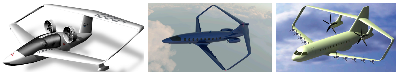
Figure 1. Artistic views of PrandtlPlane aircraft of different categories: ultra-light amphibious (left) [43], executive class (centre) [49], hybrid electric regional airliner (right) [15].
