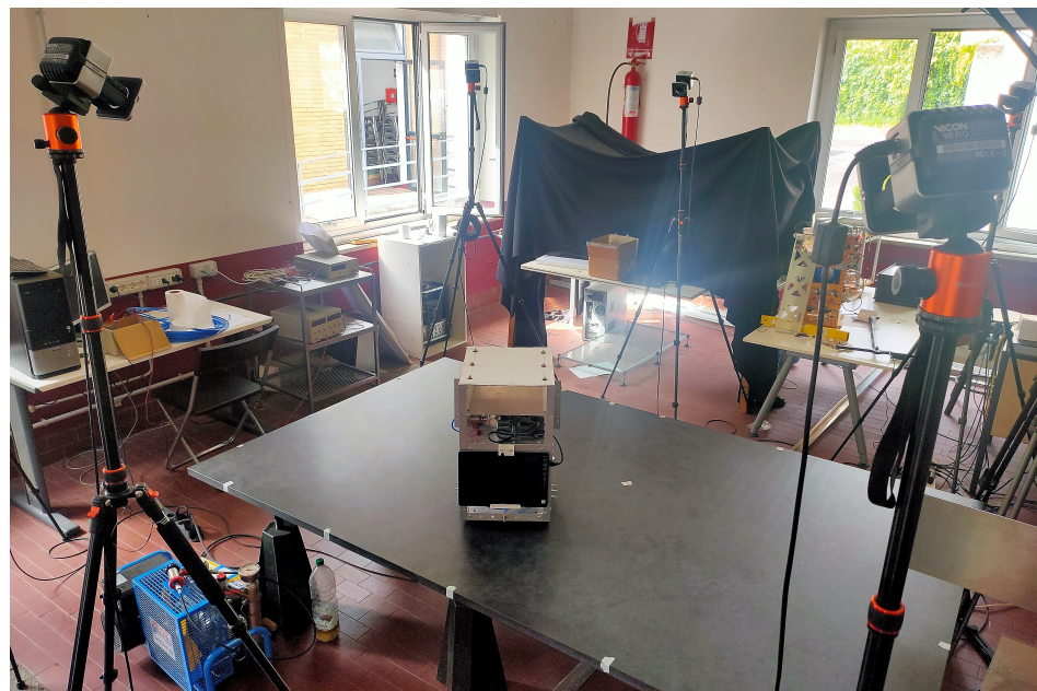
Figure 2. Photo of the PINOCCHIO platform bus on the frictionless table surrounded by the cameras of the metrology system.
