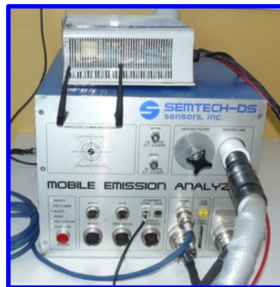
Figure 4. SEMTECH DS gaseous emission analyzer.
