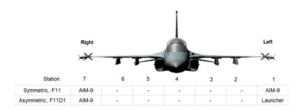
Figure 5. Test aircraft configuration.
