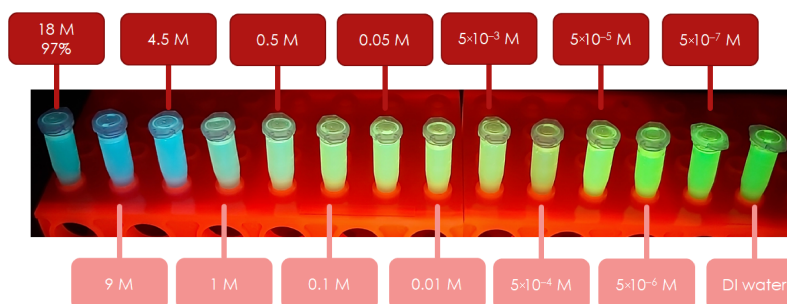
Figure 3. Fluorescein in \text{H}_2\text{SO}_4 solutions under an UV-A mercury vapor lamp with the main spectral line at 365 nm.
