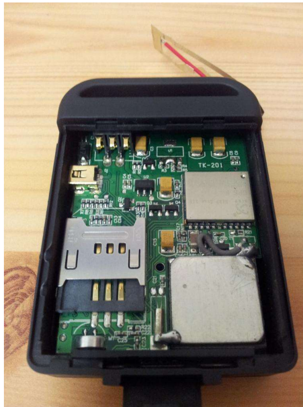
Figure 15. TK102B GPS/GSM tracker module—antenna at top.
