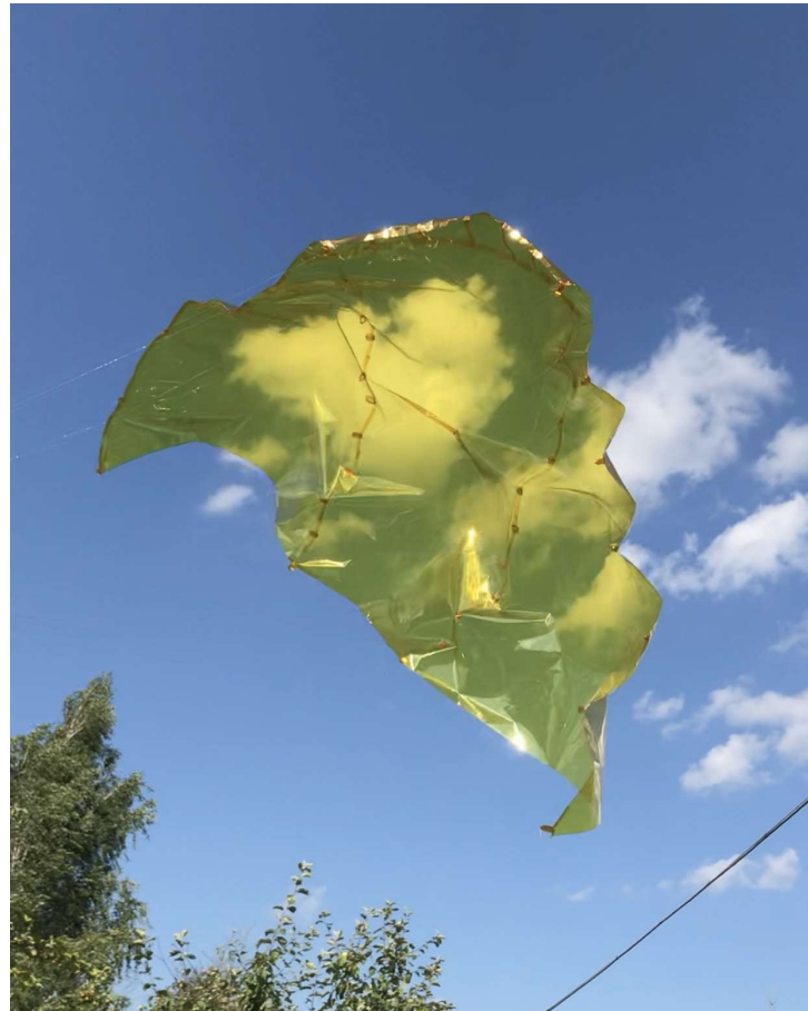
Figure 12. Prototype Kapton wing being flight-tested as a kite.
