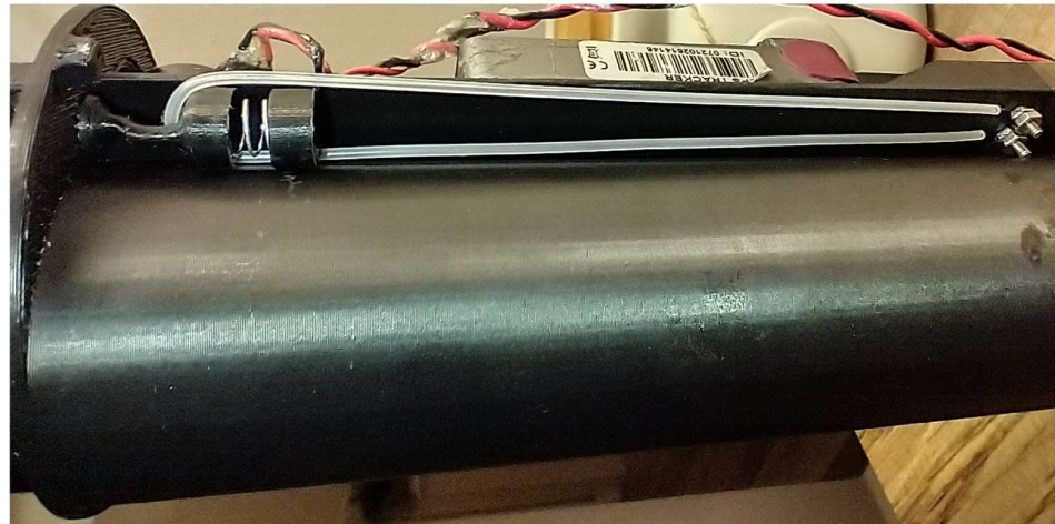
Figure 16. Shape memory alloy wire with silicone sheath.
