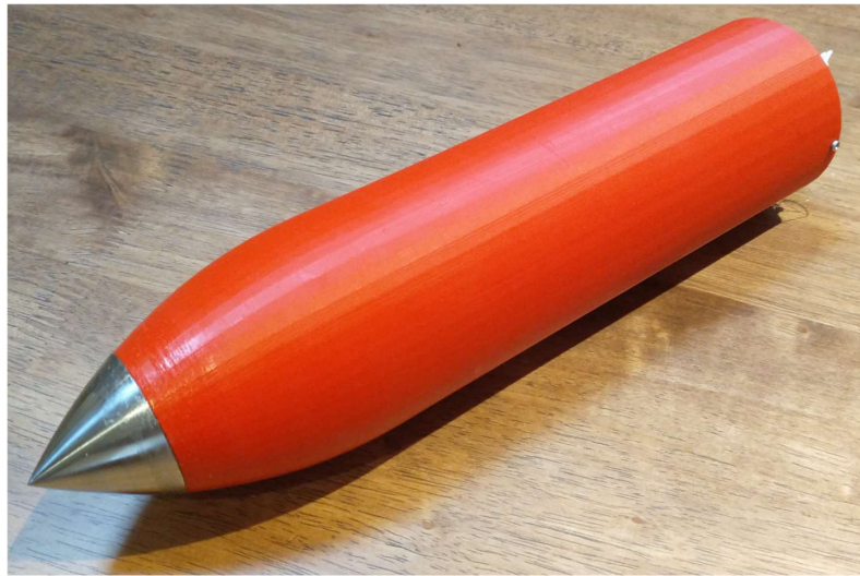
Figure 18. 3D printed casing and stainless steel tip mass.
