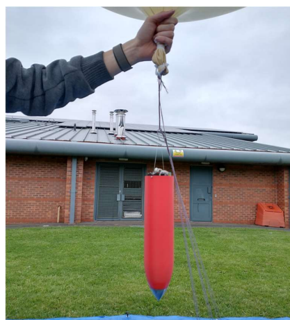
Figure 26. Capsule payload suspended beneath the balloon.
