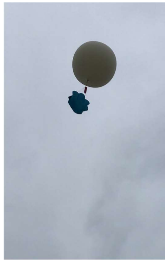
Figure 30. Balloon ascent, showing that the recovery chute (blue) was not in-line between balloon and capsule.
