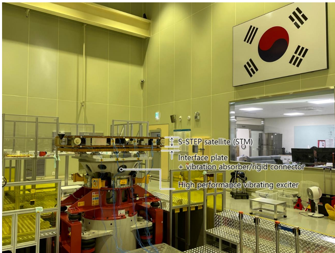
Figure 5. Experimental setup of a random vibration test for the STM of the S-STEP satellite.
