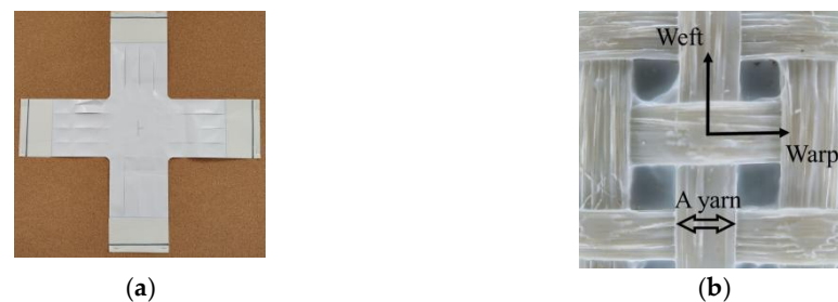
Figure 4. UN-5100 material. (a) A specimen made of UN-5100. (b) The microstructure of the UN-5100 material.
