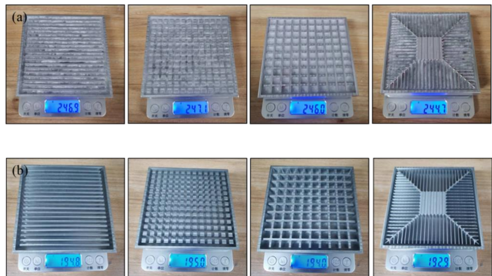
Figure 3. Weight of module (a) before PCM filling and (b) after PCM filling.
