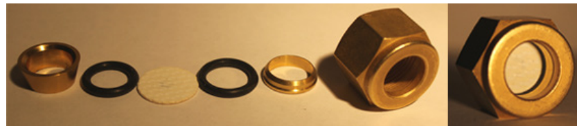
Figure 3. Assembly structure for the leak test of various material samples.
