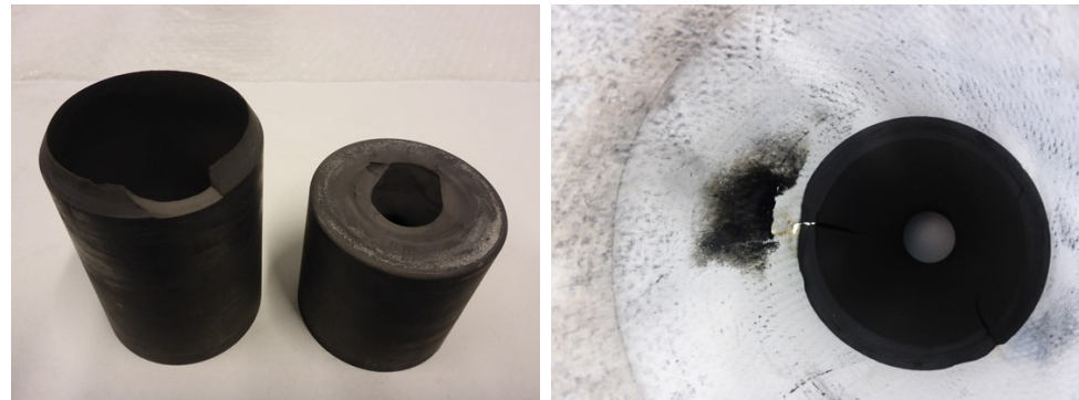
Figure 28. Damage to the graphite used in the steel combustion chamber during hot tests (left) and crack that occurred in the OCMC shell due to a local overload resulting from damage to the graphite (right).
