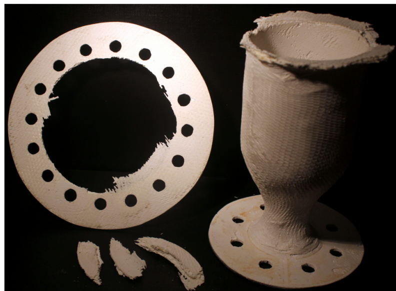
Figure 23. Prototype destroyed as a result of the pressure test with torn-off flange.
