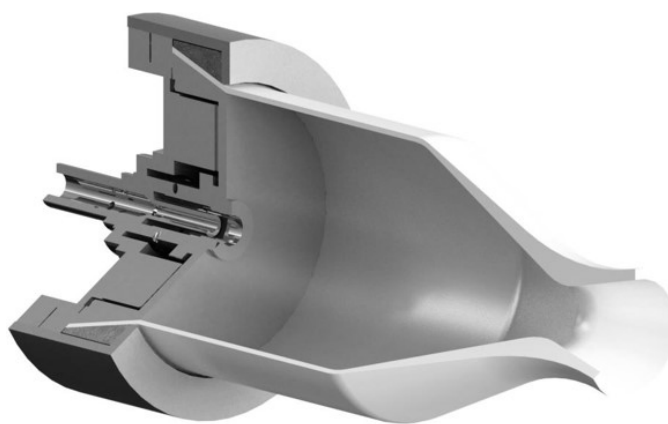
Figure 32. Revised engine design for a pure OCMC combustion chamber with nozzle.
