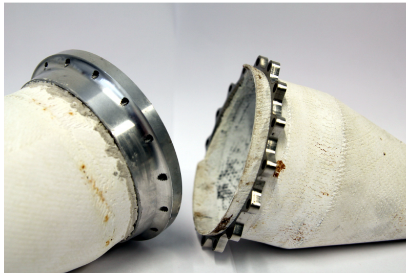
Figure 31. Comparison of the revised ( left ) with the clamping ring ( right ), which has been proven to be inadequate in tests.
