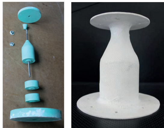
Figure 6. (left) Segmented structure of the production mould and (right) first manufactured prototype with a total mass of around 300 g.
