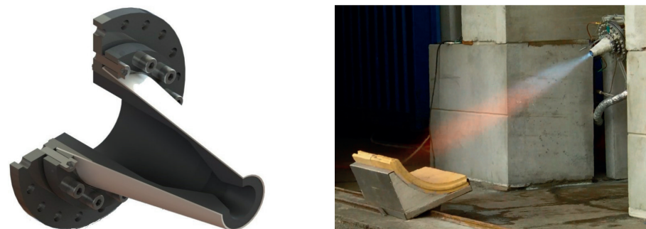
Figure 27. (left) sectional view of the OCMC combustion chamber with graphite lining and (right) its use in a hot test.
