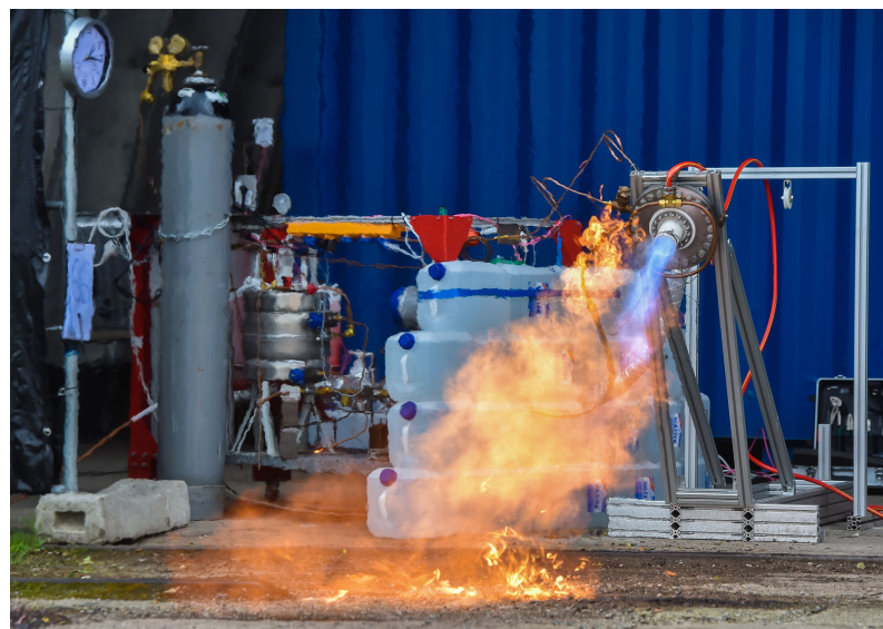
Figure 5. Hot test of the flame tube carried out with the engine test rig ©Holm Helis.
