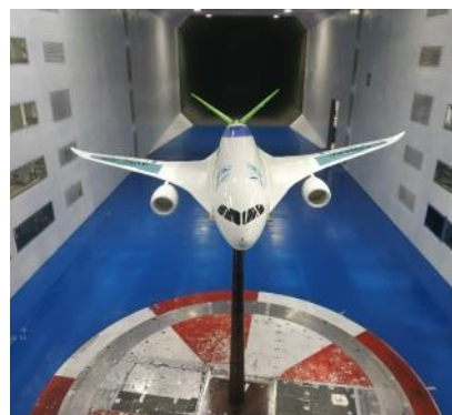
Figure 5. Installation of the model in the wind tunnel virtual flight test.
