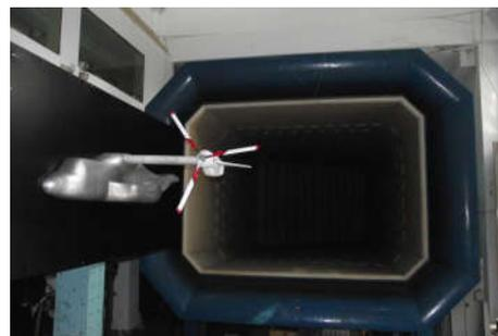
**Figure 4.** Wind-tunnel test with a scaled semi-span model.
