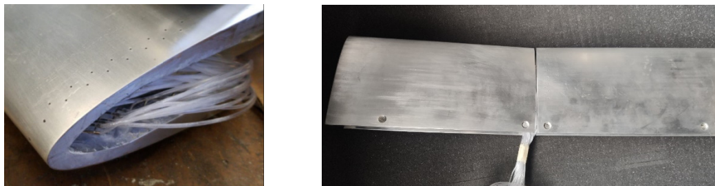
Figure 4. Pressure taps at one leading edge.
