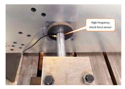
Figure 3. Shock loading device and measurement method of force signal.
