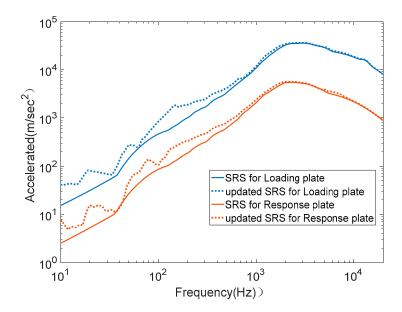
**Figure 14.** Shock response spectrum results of typical spacecraft structures based on the FRF correction and VMSS.
