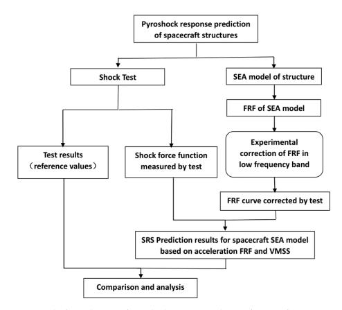
Figure 1. The frame diagram of pyroshock response prediction of spacecraft structures.
