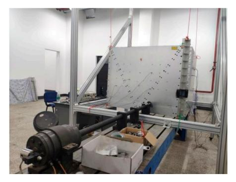
Figure 2. Shock test state of coupling plate structure.
