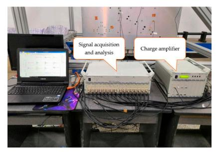
Figure 4. The measurement and control system of the experiment.
