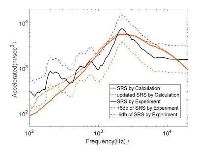
Figure 16. Shock responses of experiment and calculation for response plate.
