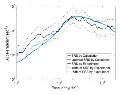
Figure 15. Shock responses of experiment and calculation for loading plate.
