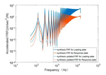
Figure 13. Synthesis FRF curve before and after correction.
