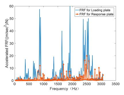
Figure 11. The FRF test results of the coupling plate.
