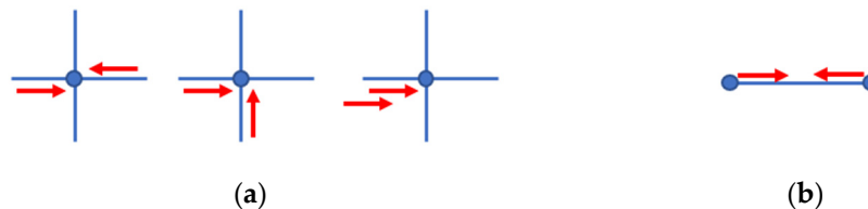
Figure 6. Two types of aircraft conflict on a taxiway. (a) 1st type conflict at each node. (b) 2nd type conflict at each edge.
