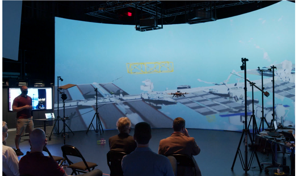
Figure 26. Onboard drone computer vision testing inside a physical/virtual simulation projection at Virginia Tech's CUBE facility.
