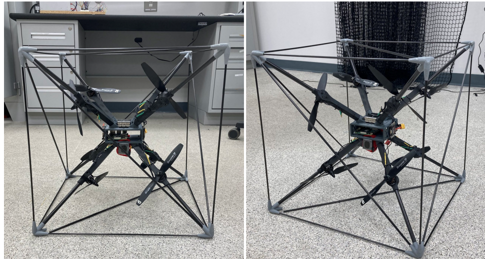
Figure 41. Virginia Tech Omni-directional drone (Omnicopter).
