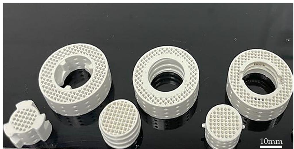
**Figure 6.** Green parts (from left to right: U-lock, Thread, Twist-lock).
