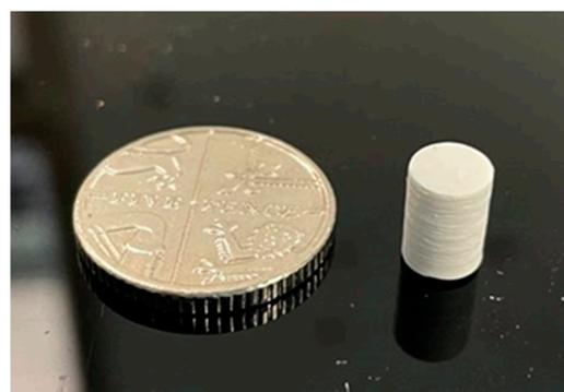
**Figure 1.** Digital Light Processed green sample.
