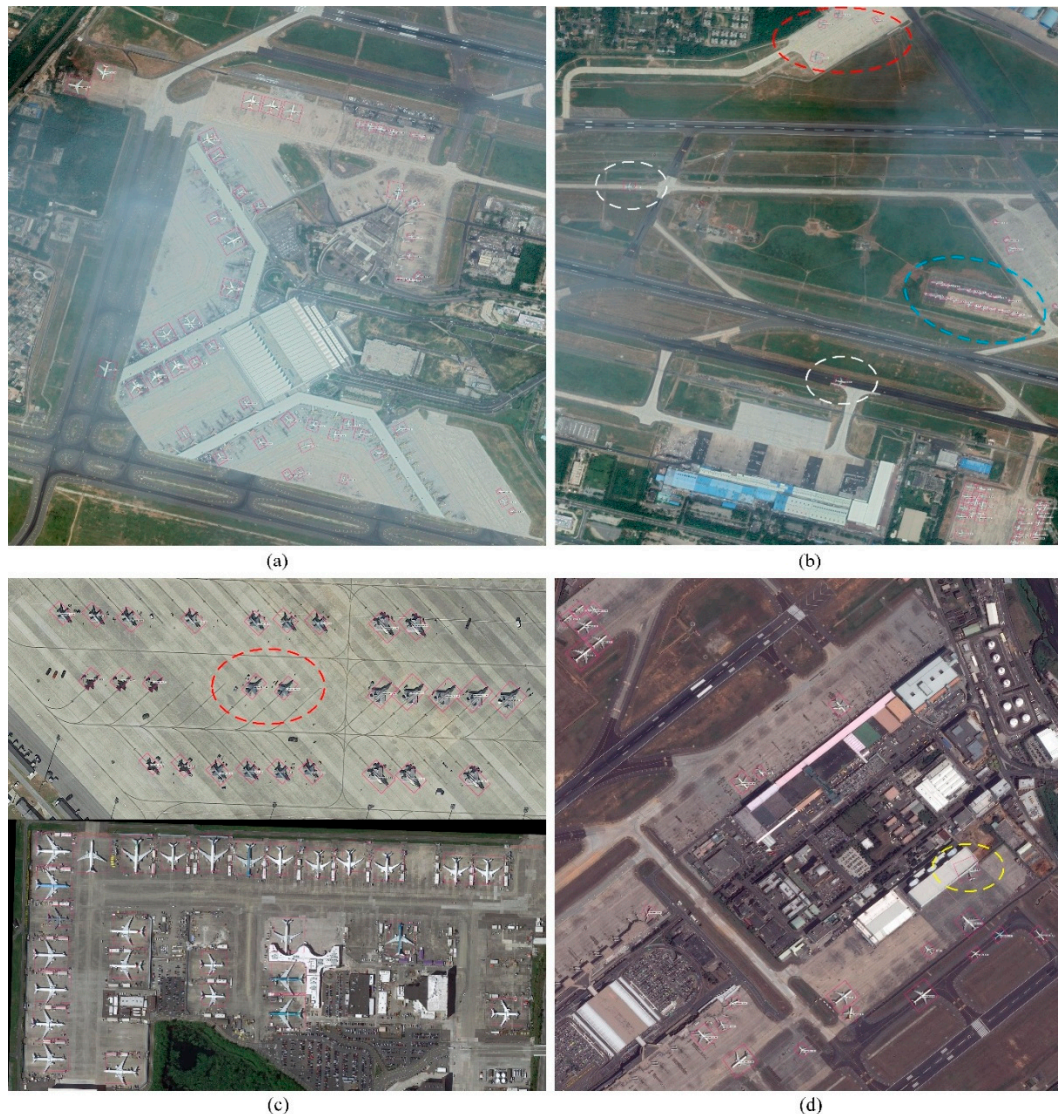
Figure 5. Aircraft detection results (confidence larger than 0.8) in test remote sensing images. (a) Aircraft detection results under thin cloud weather conditions; (b) Aircraft detection results on the apron and runway under thin cloud weather conditions; (c) Detection results of different types of military and civilian aircrafts; (d) Partially occluded aircraft can also be accurately detected.
