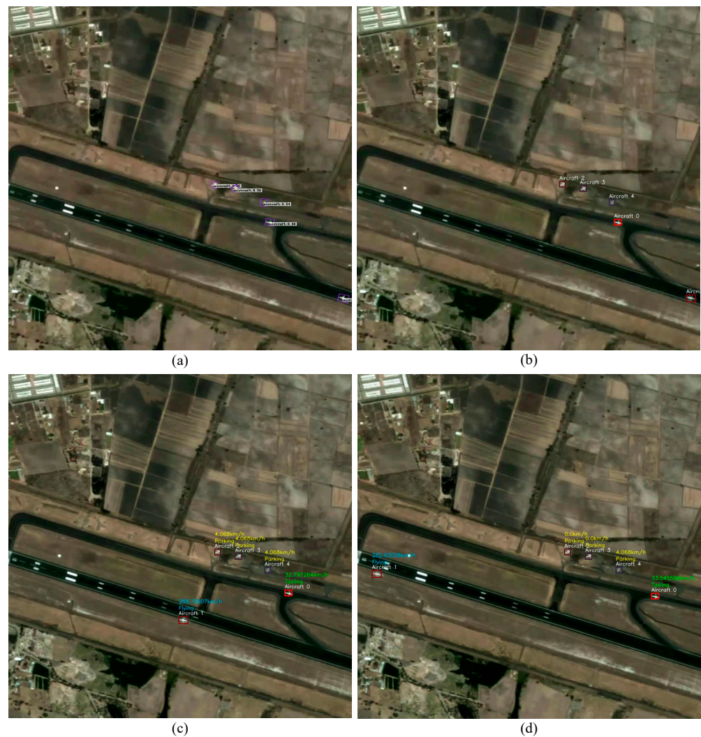
Figure 10. Screenshots of the experimental results from test Video 1. (a) Aircraft detection results in the first frame of the video; (b) Aircrafts detected in the starting frame are all tracked stably; (c) The speed of each tracked aircraft is measured and from this the type of aircraft activity is determined; (d) Each aircraft is stably tracked and its type of activity is determined.
