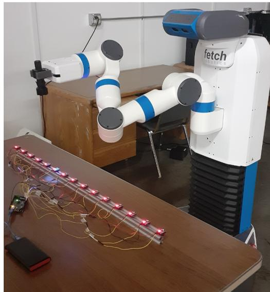
**Figure 4.** A Fetch robot hovering UV flashlight above UV sensor array.
