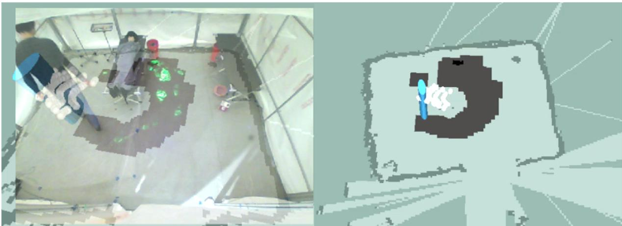
**Figure 2.** (Left): Directly detected footprints (green) and modeled areas of contamination (grey) overlaid on the camera image of the ETU. (Right): Visualization of the tracked person and modeled contamination.
