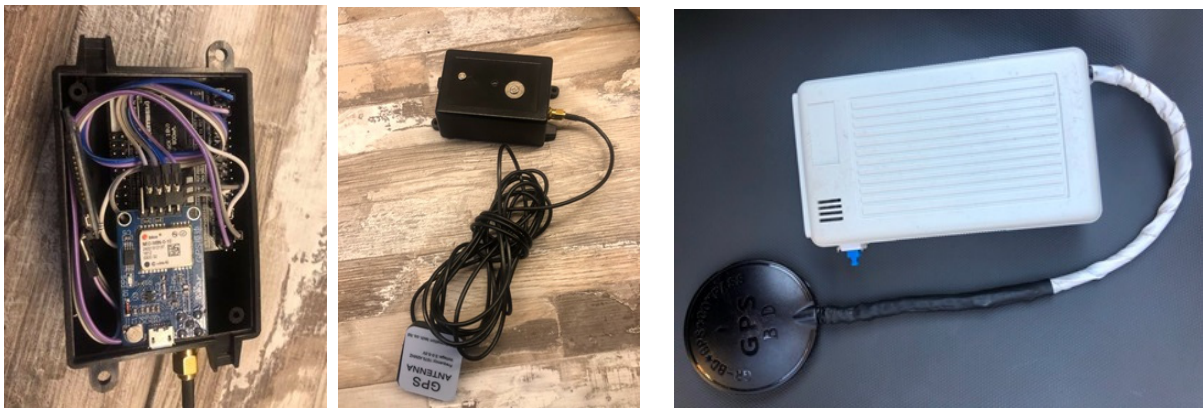
Figure 1. External wireless microelectronic device of the outdoor blind navigation application.
