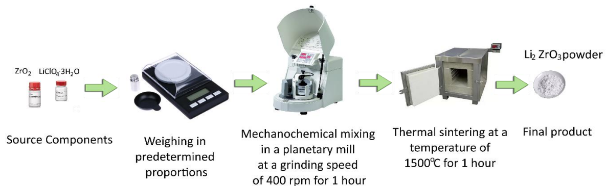
Figure 1. Schematic representation of the production of \text{Li}_{2+4x}\text{Zr}_{4-x}\text{O}_3 ceramics.
