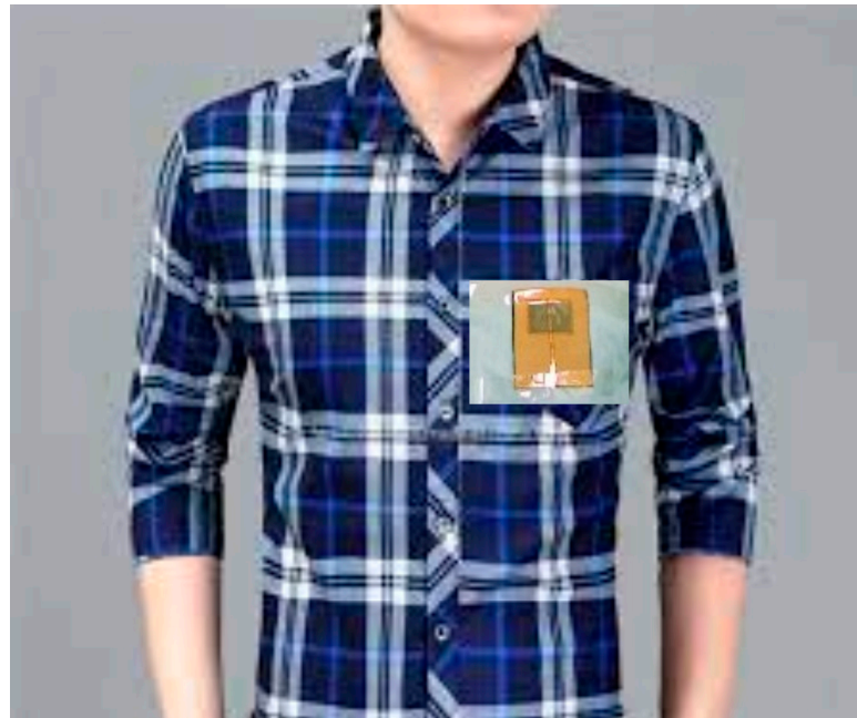
Figure 1. A clumsy, wearable patch antenna attached to a shirt with a plastic, transparent sheet; computer simulation based on [6].
