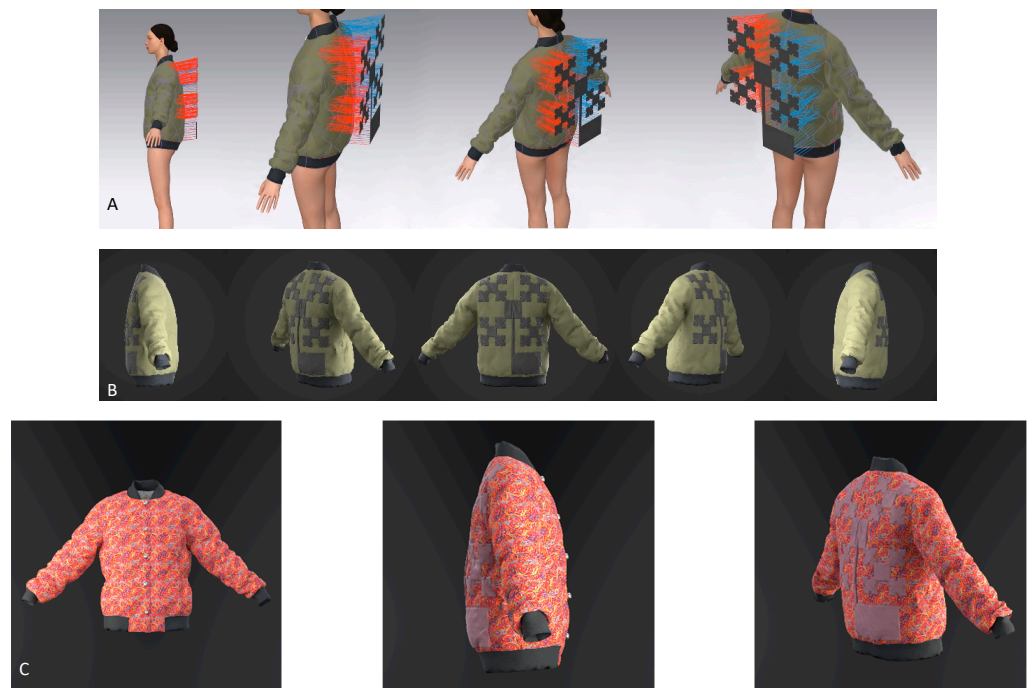
Figure 7. A third-order Minkowski fractal antenna integrated into a women's bomber jacket.
