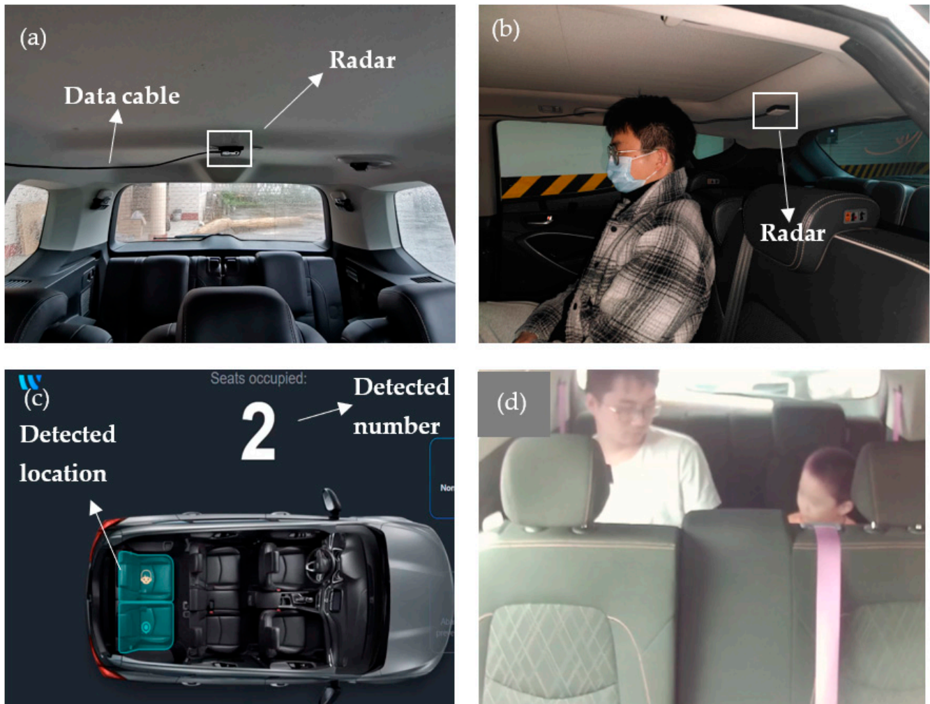
Figure 12. Radar placement and experimental environment: (a) front view of the radar mounting position; (b) left view of passenger and radar; (c) the interface where the results are presented. Where the number of people is marked in the upper part and the location of the passengers are marked in the vehicle (d) live in-vehicle view of the test case with one adult and one child in the third row.
